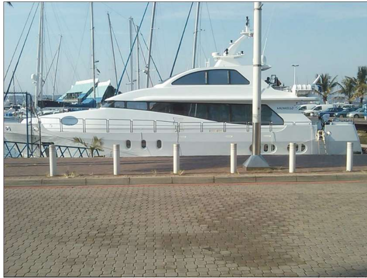
Christo an Karien's Luxury Yacht which took them five years to build and cost R46 million. It is powered by twin turbo 1050 horsepower diesel engines with ZF gearboxes. It is 90 foot long and weighs 130 tons. It carries 28 000 litre of diesel.
